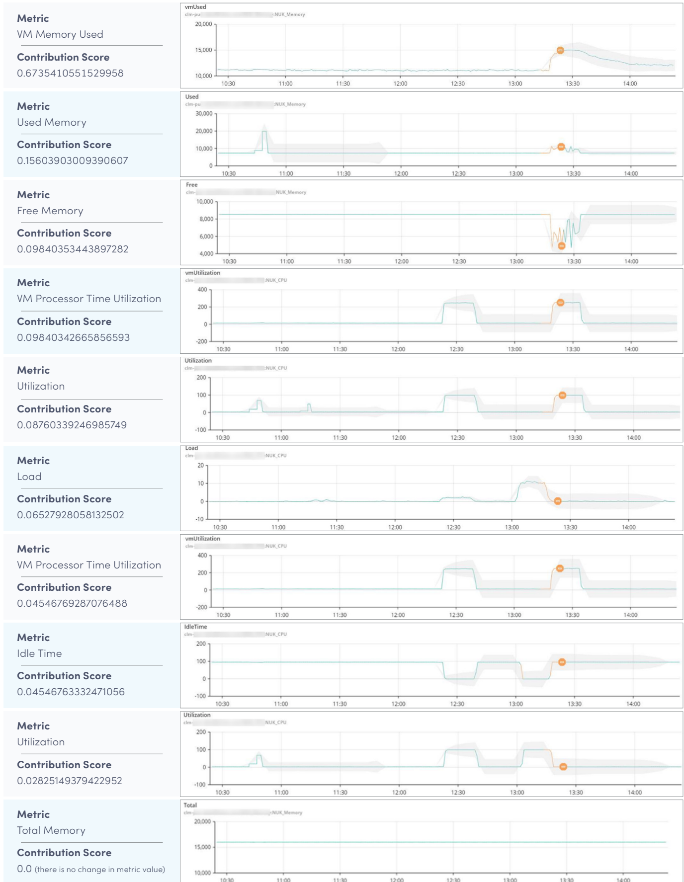
Figure 15: The table above lists how each metric has contributed to the anomaly score in order of most impactful to least impactful
